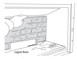
Figure 19. Install Lower Rear Panel.
